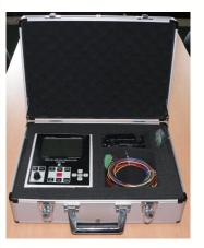
Through a collaborative consultation process, Omnitronics created the Digital Train Motion Simulator which allows for Warehouse Testing of the GCPs.
